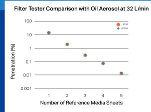
As shown in this example, the two tester models agree very well for penetration testing of flat sheet media. An increasing number of sheets is used to cover a wide range of measured penetrations.
