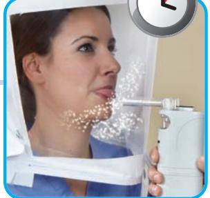
Repeat a total of three times. If no taste is detected after three attempts, the subject cannot detect the solution. Use another type of solution or another type of fit test.
