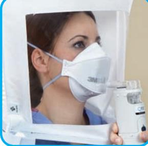
Hold the pump to the hood opening for the 7-minute fit test and activate Qfit based on the timing protocol from Table A.
