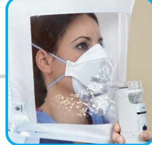
Insert the Qfit nebulizer nozzle into the hood opening for the 7-minute fit test.
