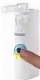
Push and hold the test button for more than 1 second to activate Qfit for each 6-second dispersion.
