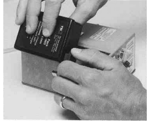
Figure I-6. Plugging in the battery connector
