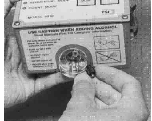
Figure X-3. Removing the alcohol fill cap
