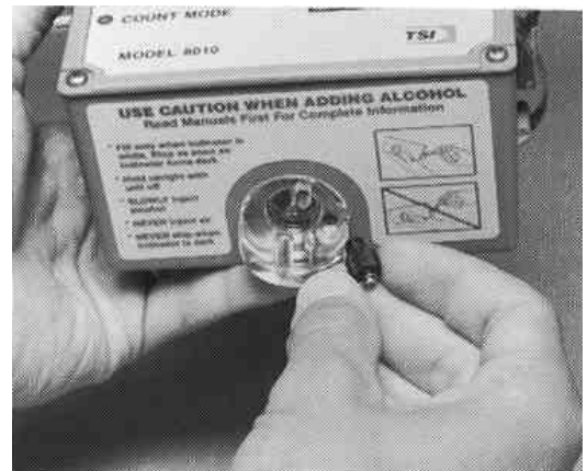
Figure I-10. Removing the alcohol fill cap
