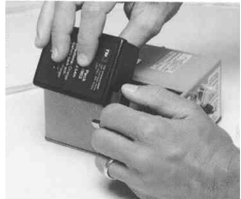
Figure X-10. Plugging in the battery connector
