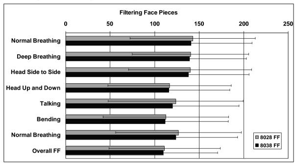
Twenty eight multi exercise Fit Tests were carried out on a sample of seven different FFPs that are commercially available in North America. Each Fit test consisted of seven exercises yielding a sample population of 196 data pairs. Again, the absolute numerical Fit Factors are not the primary subject of this comparison.
