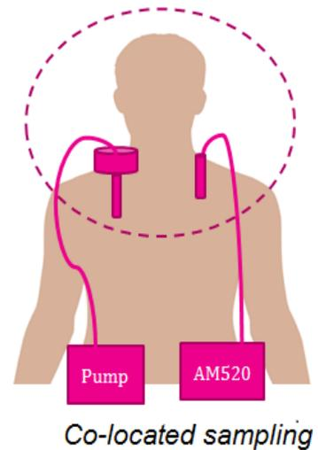
**Gravimetric Sample Pump:** The gravimetric sample is collected via a sample pump with a collection filter that is sent to an accredited laboratory for analysis. The lab will provide a report of the analysis that contains the following information:
