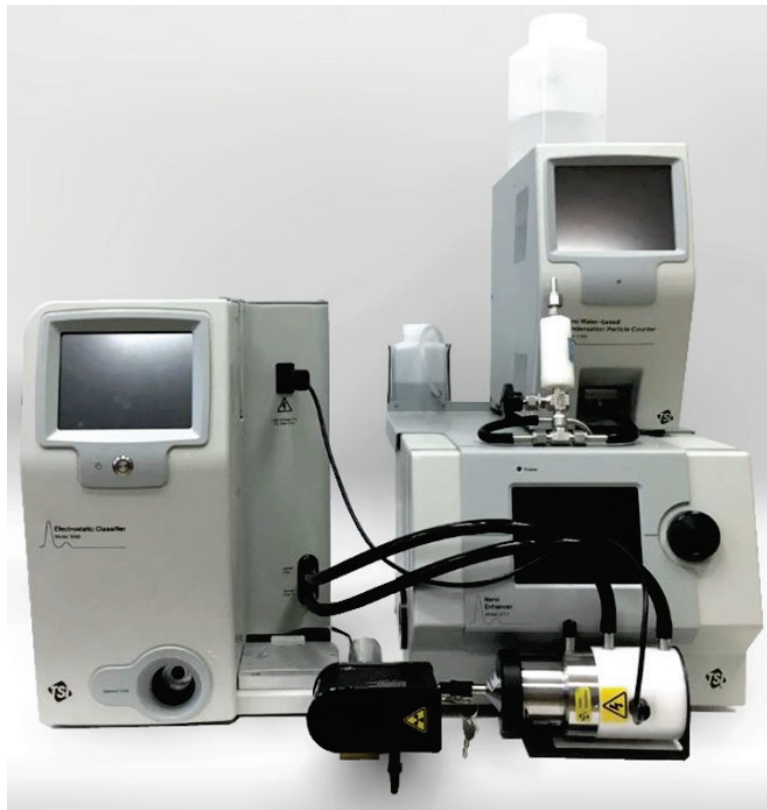
Figure 2: A 1nm SMPS system using a Model 3788 water-based CPC in place of the standard Model 3772 butanol-based CPC. The white filter and needle valve depicted in front of the Model 3788 allow makeup air into the Model 3788 when it is operated at 1.5 L/min. This allows the Model 3777 to operate at its designed inlet flow rate (details are explained below).
