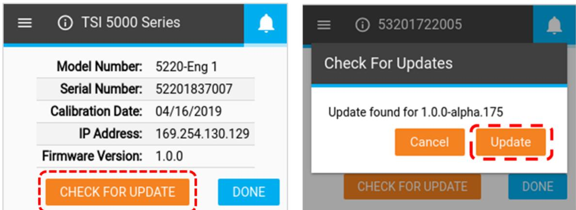
Please allow up to several minutes for the meter to update its firmware. Once complete, an **“Update Successful!”** message will display briefly and the meter will automatically reboot. After reboot the meter will be ready for operation. If the meter does not initialize after the firmware update, an additional instrument reboot may be necessary.
