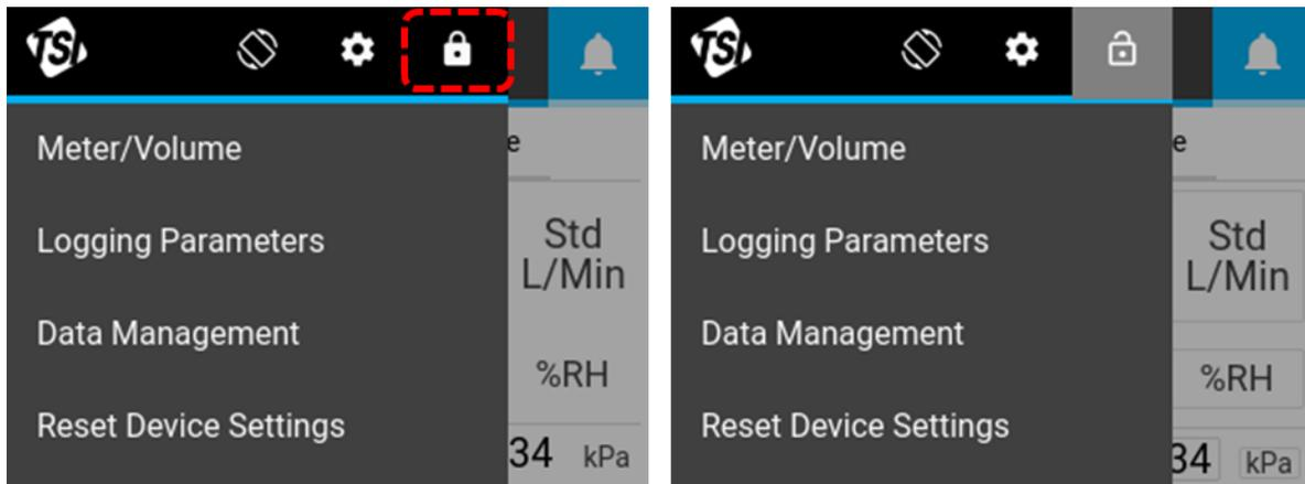
With the meter unlocked, navigate back to the Meter Home Screen by selecting **Meter/Volume** from the menu. The fields unlocked for configuration on the Meter Home Screen will have a gray box displayed around them.
