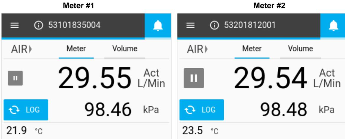
Back pressure is introduced upstream of the valve. The increased pressure of air being measured by Meter #1 causes the volumetric flow reading to decrease. Meter #2 does not experience an increase in pressure and its flow reading remains steady. The remote flow measurement is taken upstream of the valve and is consistent with the volumetric flow reading from Meter #1 at the same location in the line.
