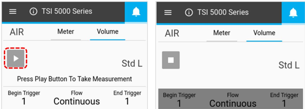
Once the **Play** button is pressed to take measurements, the Flow Multi-Meter will notify you on screen when the Begin Trigger, and then End Trigger, is reached. After the end trigger is reached, the meter will display the calculated volume measurement.
