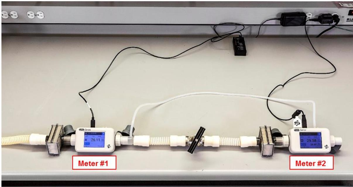
With similar temperature and pressure conditions, the volumetric flow rate between the two measurement points is consistent.
