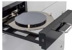
All versions can support deposition on 200mm and 300mm wafers
