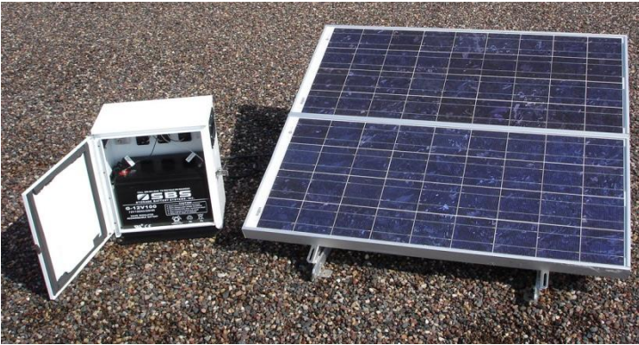
Figure 29: Solar Cell Power System
