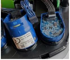
Figure 40: Remove sensor body
