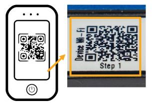
Figure 9: Scan QR code to connect to Wi-Fi®
