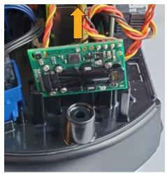
Figure 42: Lift sensor board to remove it
