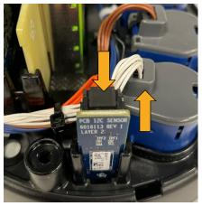
Figure 43: Disconnect sensor cable
