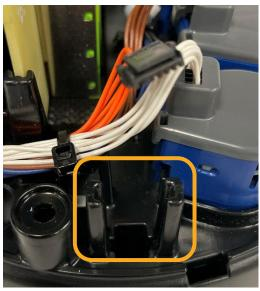
Figure 45: Reconnect cable connector
