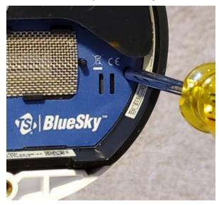
Figure 34: Remove cover screws
