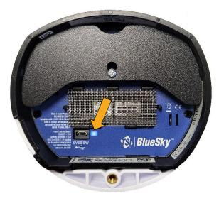
Figure 15: Connections made – LED solid blue
