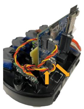
Figure 41: Disconnect sensor cable
