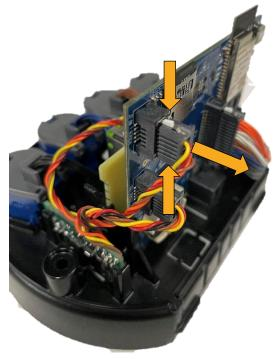
Figure 35: Disconnect cable from main board
