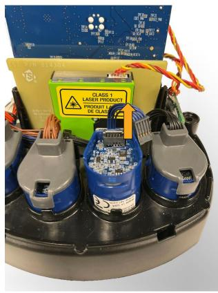
Figure 39: Disconnect sensor cable
