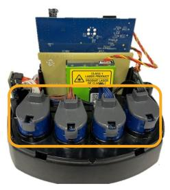
Figure 38: Replace electrochemical sensors
