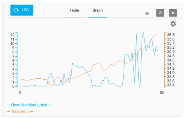
The two values present at the beginning and end of the *X*-axis show the time (in seconds) of the data that is currently displayed in the graph. For example, a data rate of 500 ms would graph 2 data points per second and the graph window would display 50 seconds worth of data (100 total readings).
