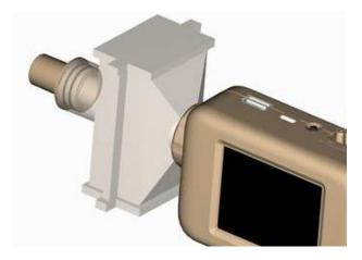
If the 0.5 inch or 15-mm tube ends are connected directly to the instrument, select the "Using 0.5 inch or 15 mm ends" Toggle Switch in the Meter's Settings screen.
