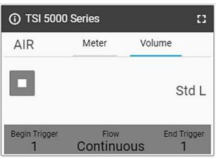
With the **Play** button is pressed and flow is occurring, the Flow Multi-Meter will notify you on screen when the Begin Trigger, and then End Trigger, is reached. After the end trigger is reached, the Meter will display the calculated volume measurement.
