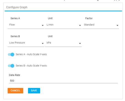
Graphing defaults to Auto-Scaling for both series on the graph. To set a custom *Y*-axis, click the slider to the left and input any numerical value into the Min and Max fields.
