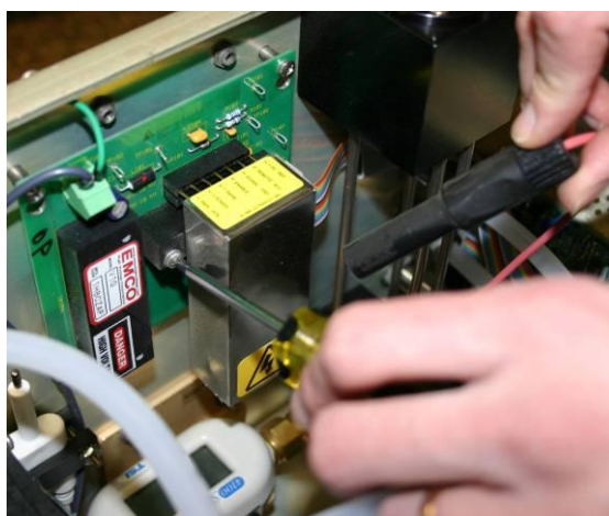
Figure 4. Removing Power Supply
