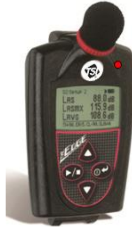
Figure 1-1: Sample measurement display
