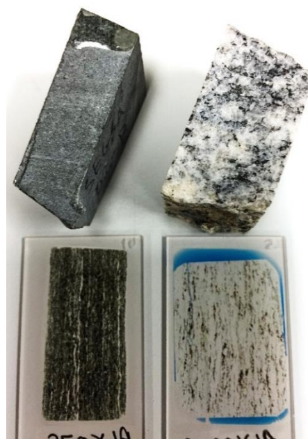
Figure 2. Feldspar rock samples, raw and prepared on microscope slides.
