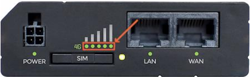
Figure 6: Signal strength LEDs
