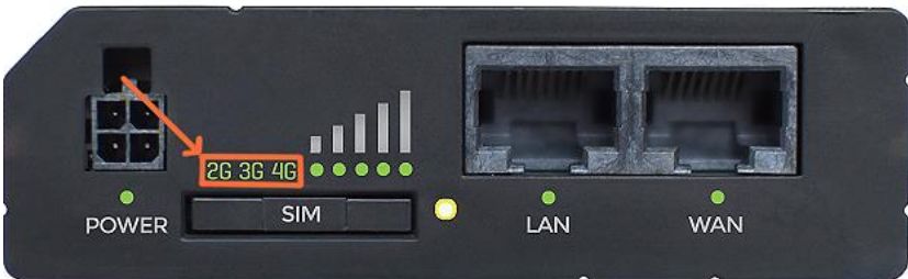
Figure 5: Connection status LEDs
