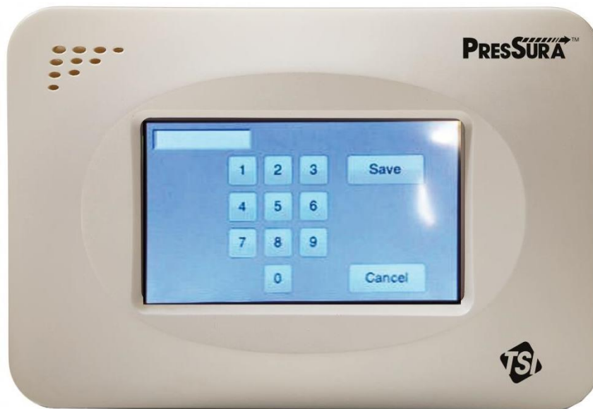
Figure 37. Access Code Screen
