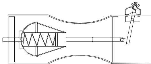
**Note:** *If the valve is configured and calibrated for horizontal or vertical operation, the valve must be level when mounted in the ductwork to operate precisely.*
