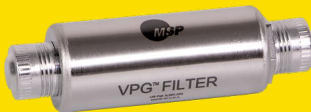
Conventional high-purity, point-of-use gas filters are used in a compressed gas line for particle removal. The VPG-A3 filter is also used downstream of a vaporizer under vacuum flow conditions to prevent particles, which could potentially be in the gas/vapor mixture, from entering the Chemical Vapor Deposition (CVD) or Atomic Layer Deposition (ALD) process chamber. The VPG-A3 filter is made from 316L SS sintered powder media and has a large surface area, giving the filter a long lifetime.
