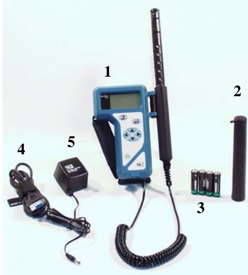
Figure 1-1: Models 8552/8554 Q-TRAK Plus IAQ Monitor with Calibration Collar and Batteries
