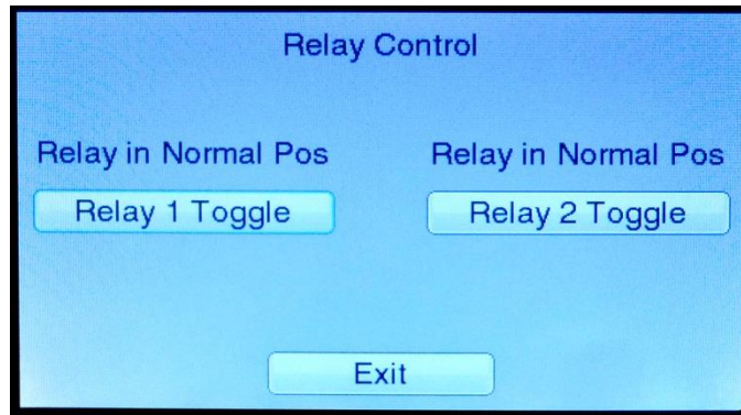
Figure 16. Relay Outputs screen in Diagnostics menu
