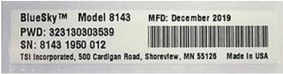
Figure 8: Security Key (PWD) location
