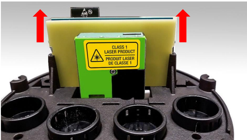
Figure 27: Replacing PM sensor
