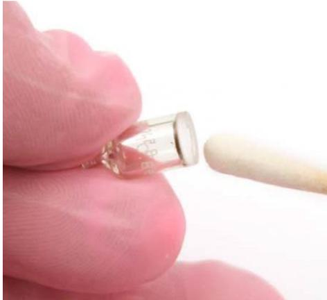
**Figure 30: Polishing the Electrode Lamp Window**
