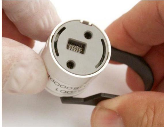
**Figure 36: Using Removal Tool**
