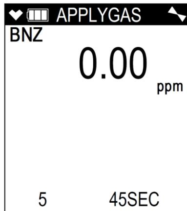
12. At the end of the countdown, use the **▲ AIR** or **SHIFT ▼ (PANIC)** button to adjust the reading to match the concentration listed on the calibration cylinder.
