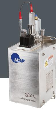
MSP's 2841PE Turbo™ Vaporizer was designed for high flow microelectronic applications. It has the state-of-the-art Performance Enhanced (PE) atomizer with on-board flow control and dual heaters to compensate for evaporating cooling at high liquid flow.
