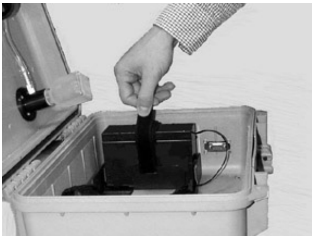
Figure B-12: Tighten Velcro Around Battery.
