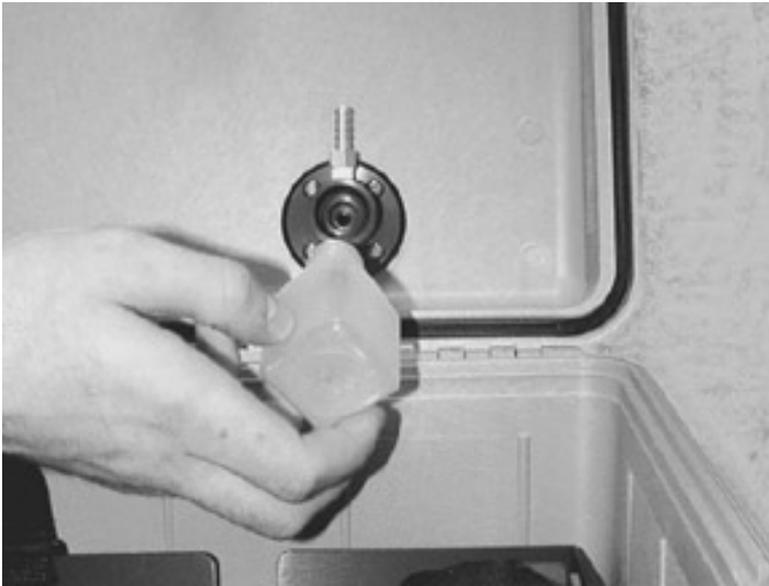
Figure B-5: Installing the Water Trap Bottle
