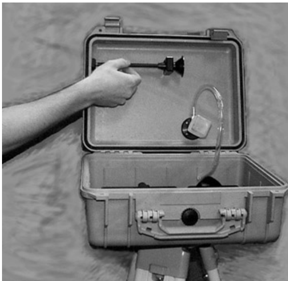
Figure B-3: Unscrew Inlet from Inner Bracket
