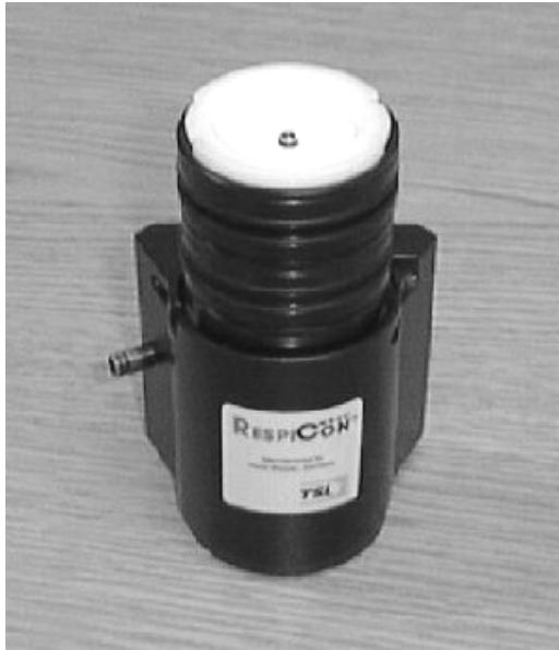
Figure 2-5: Place Body Unit Over Removal Cylinder. Place Stacked Filter Stages into Body Unit.
