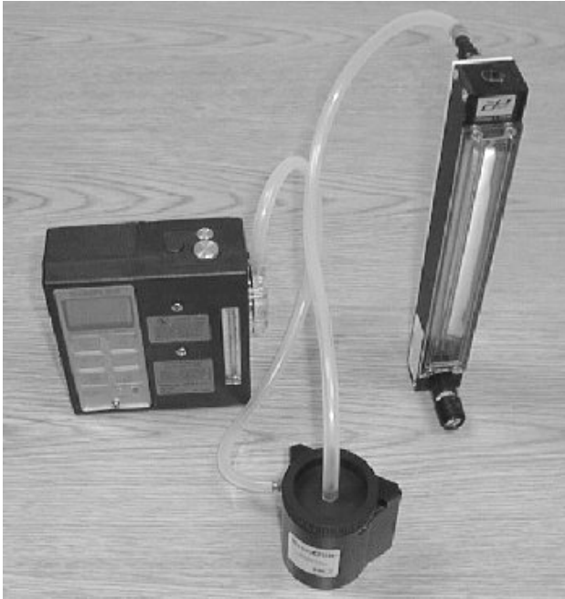
Figure 4-4: Attach Flowmeter and Sampling Pump to RESPICON Total Flow Checker 1
