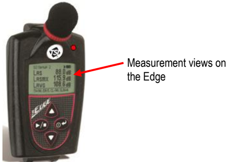
Figure 4-9: Measurement view on the Edge
