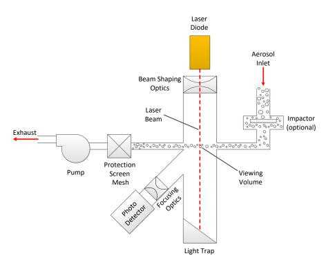
an internal calibration constant to yield factory calibrated mass concentration. The internal calibration constant is determined from the ratio of the voltage response of the SidePak™ AM520/AM520i monitor to the known mass concentration of the calibration test aerosol (A1 Test Dust).
