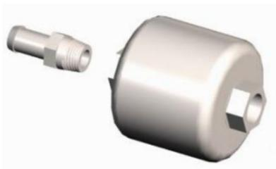
3. Connect outlet side of the Filter to inlet side of 3/8 inch NPT Tube End.
