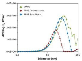
Figure 5. The volume distribution of engine emissions as measured by an SMPS, and by the EEPS™ using two data inversion matric
