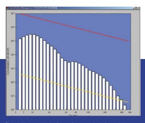
Figure 8. Histogram showing "in-range" concentration indicators (minimum in yellow; maximum in red). Log scale makes it easy to see nucleation and accumulation modes.
