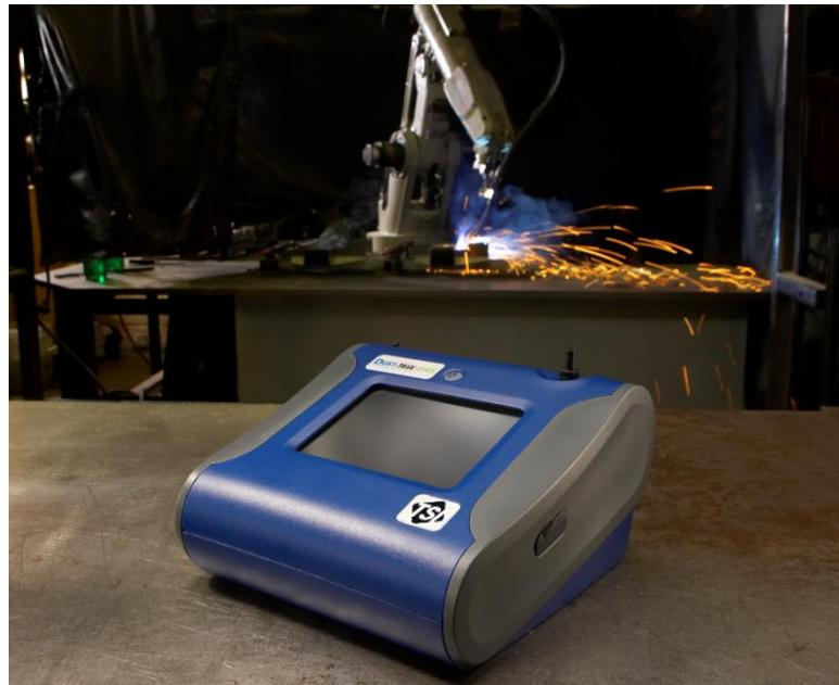
When the welding set up is changed, the DustTrak Aerosol Monitor readings are checked to verify the ventilation controls are properly positioned to control welding fume at the point of generation to minimize fume buildup in the shop. The portability of the DustTrak Aerosol Monitor facilitates using the instrument to spot check specific workstations and troubleshoot areas with higher aerosol concentrations.
