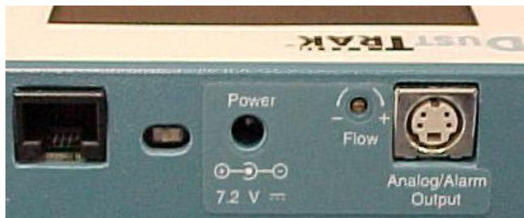
**Note:** For technical information on using the DUSTTRAK<sup>™</sup> monitor's analog output features see [Application Note ITI-074, Analog Output](#) on the TSI Website at [www.tsi.com](http://www.tsi.com).
