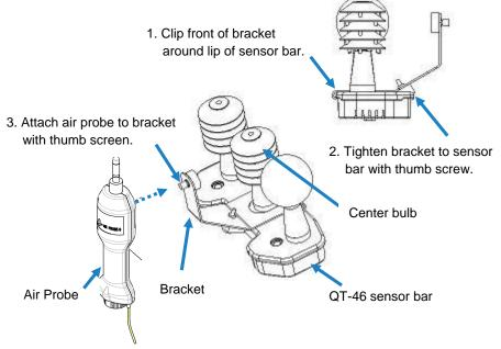
Figure 27: Air flow configuration
