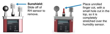
Figure 22: Sunshield & placement of finger cot prior to RH verification
