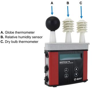
Figure 5: Sensors identified
