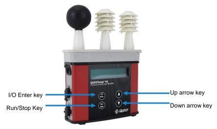
Figure 2: Keypad explained and identified
