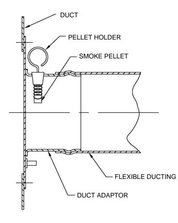
As shown in the sketch a rubber bung is fitted into the hole in the duct adaptor which holds the wire coil.
