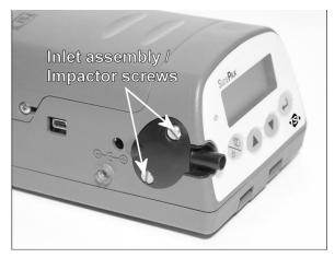
2. Use a small screwdriver to push against the flange on the insert stem and slide the insert out of the impactor body.
