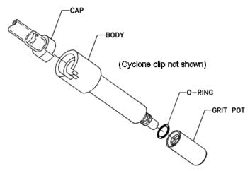
Exploded View of 10 mm Nylon Dorr-Oliver Cyclone
