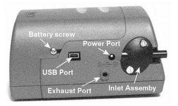
The power supply cannot run the SidePak monitor and charge the battery at the same time. Make sure the instrument is off to facilitate charging. If the display does not show CHARGING BATTERY, it is **not** charging.
