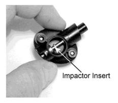
To make sure unwanted (large) particles remain trapped on the insert, it is necessary to apply a small amount of impactor grease (vacuum grease) for the particle to stick to. Grease is also applied to the O-rings to aid assembly and improve sealing.
