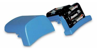
Install six AA-size battery cells. Make sure the cells are installed in the proper direction by matching the polarity markings on the cell holder with the markings on the battery cells.
