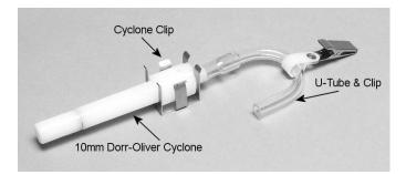
Four micrometers (4  $\mu$ m) is internationally accepted as the 50 percent cut-off size for respirable aerosols. Particles larger than 4  $\mu$ m impact onto the surfaces of the upper respiratory tract and cannot reach the lungs. The cyclone accessory provided with SidePak AM510 kits is designed to provide a cut-off at 4  $\mu$ m. This is specified as a 50 percent cut-off at 4  $\mu$ m.
