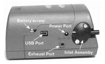
The power supply cannot run the SidePak monitor and charge the battery at the same time. Make sure the instrument is turned off to initiate the charging cycle. If the display does not show CHARGING BATTERY, it is **not** charging.
