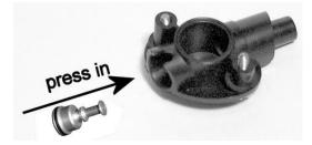
6. Screw the impactor assembly back onto the AM510 body and tighten the two captive screws. Do **not** over tighten.
