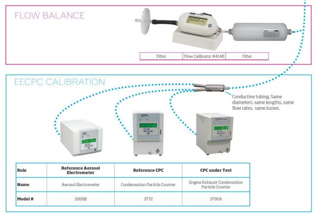
Figure 1: Schematic of the EECPC Calibration Setup
