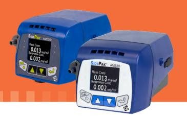
The SidePak<sup>™</sup> AM520 and AM520i Personal Aerosol Monitors are small, portable, battery-operated, data-logging, light-scattering laser photometers that provide real-time aerosol mass concentration readings of dusts, fumes, mists, smoke and fog within a worker's breathing zone.
