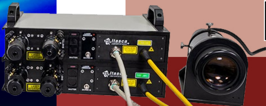
System layout of a 2D Itasca-based PDPA System with FSA Signal Processor
