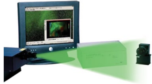
2D PIV system with a single camera and laser for planar 2D velocity field measurements.
