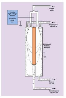
Figure 2. Operation principle of the DMA
