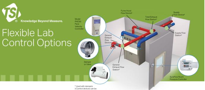
‡ Control devices can be dampers or venturi valves
