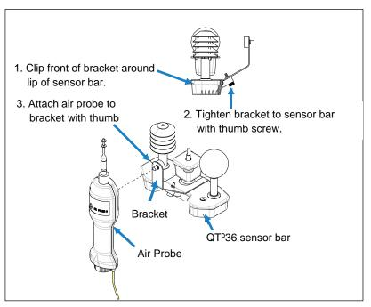
Figure 21: Air flow configuration
