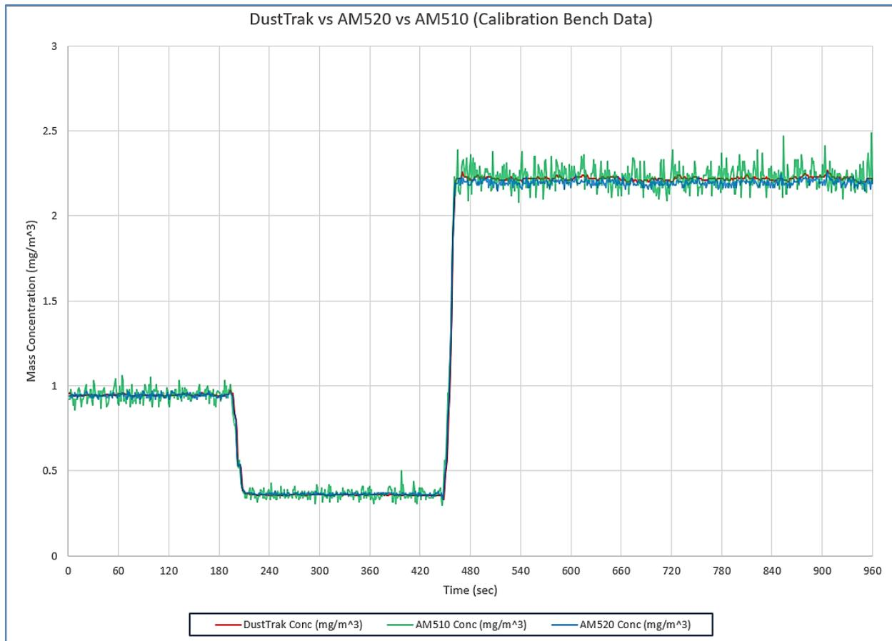
As the graph above shows, each instrument will have a unique response signature to the same aerosol, with the SidePak AM510 showing the most variability. However, the correlation of all three instruments are very similar with the DustTrak II monitor and SidePak AM520 being very closely aligned.
