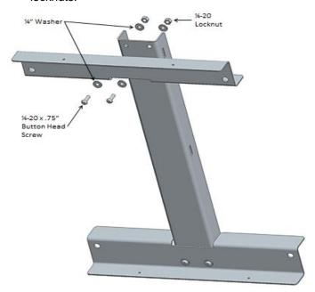
Attach the pole mount to 4 locations on the environmental enclosure using the provided 3/8" screws, washers, and nuts.
