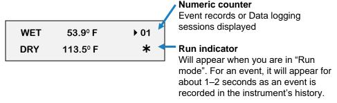
Figure 7: Measurement screen (example)
