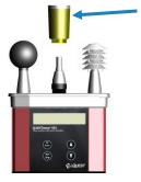
Alignment salt (remove rubber cap and place over RH sensor with the sunshield removed)
