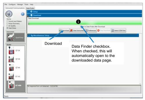
Figure 33: Communicating with the QT<sup>0</sup> 48N and DMS
