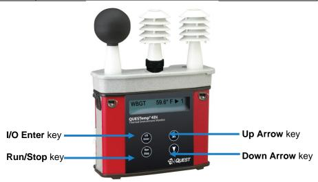
Figure 2: Keypad Keys identified
