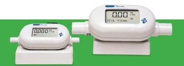
TSI offers two Primary Calibrator Models for calibrating pumps and any other air sampling instruments that draw an active air sample. These small, portable, battery-operated units are lightweight and easy to use. Volumetric flow rate is displayed continuously, making real-time pump adjustment, calibration and periodic flow checks fast and easy. These Primary Calibrators are temperature-compensated and pressure-corrected to calculate volumetric flow rate at an accuracy within 2% of reading.
