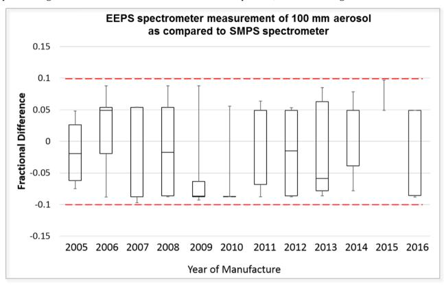
**Figure 1:** EEPS instruments' measurement of 100 nm classified aerosol, compared to SMPS spectrometer measurement of the same aerosol, grouped by year of manufacture. The oddly shaped plot for 2015 is due to the fact that 92% of EEPS instruments manufactured that year deviated from SMPS measurements by the same value,  $\sim$  5%. The dashed lines represent  $\pm$ 10%, TSI's internal requirement for EEPS–SMPS agreement.
