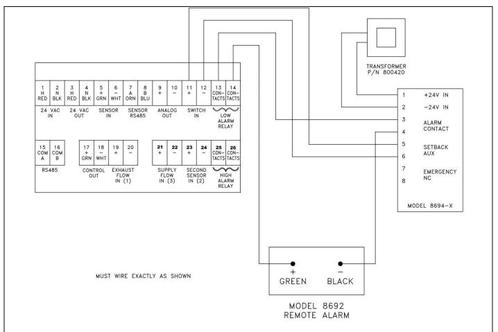
**NOTE:** Use Figure 2 if using one Digital Interface Module to one Model 8692 Remote Audible Alarm and one Model 8694 Remote Alarm.
