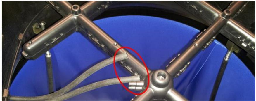
3. The short tubing ends can be inserted into the pole support bracket to keep them out of the way.
