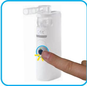
Push and hold test button until yellow LED light turns on.
