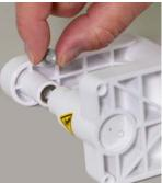
Step 4: Use the PortaPunch™ Probe Insertion Tool (with probe loaded) to puncture the respirator from the inside. It is not necessary to push the probe all the way through. All you need to do is get the point through far enough to be seen from the other side.
