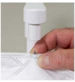
**Step 5:** Next, press down on the PortaPunch<sup>™</sup> lever arm to engage the push nut onto the exposed point poking through the respirator and firmly push them together as far as possible.
