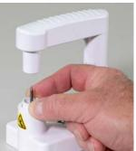
**Step 3:** Load a push nut onto the magnetic push nut tool on the PortaPunch™ tool.
