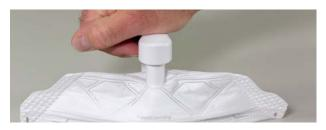
Step 6: Release the PortaPunch™ lever arm and remove the respirator and inspect the sample port to make sure it is tightly secured and will not leak. You should not be able to rotate the probe with your fingers. If necessary, use the PortaPunch™ Probe Insertion Tool again to tighten the port.
