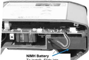
To install: Slide into case and plug in connector as shown.
